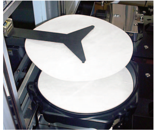
Entegris multilayer nonwoven inserts are transferred into a 300 mm SmartStack horizontal wafer shipper by the Cybernetix WPC300 tool.
